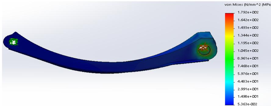
**Fig. 9.** Von mises stress for the existing Rear Trailing Arm of 1G bump load
