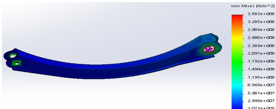
**Fig. 10.** Von mises stress for the existing Rear Trailing Arm of 2G bump load
