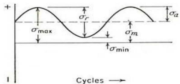
Fig. 18. Repeated stress cycle
