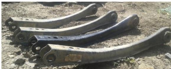
**Fig.1.** The existing damaged rear trailing arm
