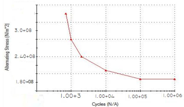
Fig. 19. Alternating cycles vs. number of cycles for the existing Rear Trailing Arm
