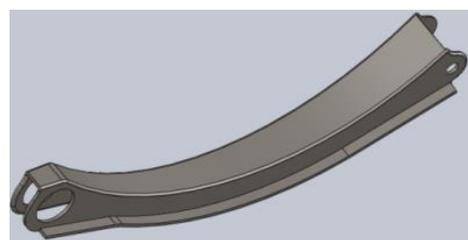
**Fig. 3.** 3D Modeling and 2D drawing of the original trailing arm
