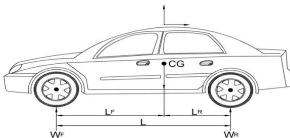
**Fig.7.** Free body diagram of Geely Addis Automobile
