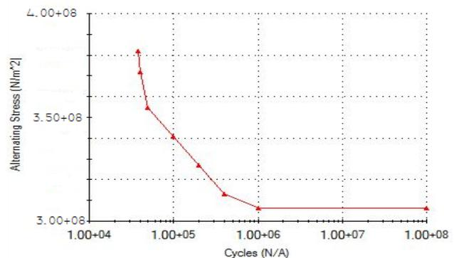
Fig. 20. Alternating cycles vs. number of cycles for the modified Rear Trailing Arm
