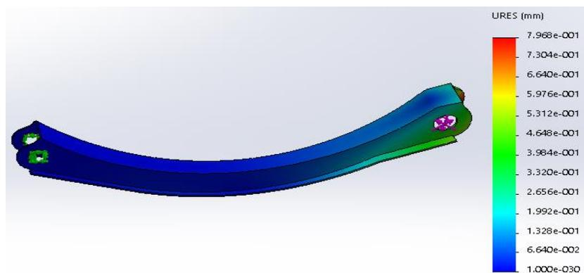
Fig. 13. Deformation for the existing rear trailing arm of 2G bump load
