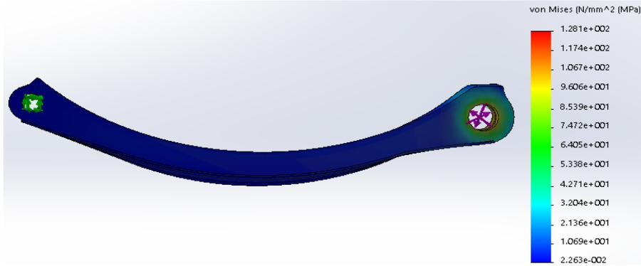
Fig. 15. Von Mises Stress for modified design of Rear Trailing Arm
