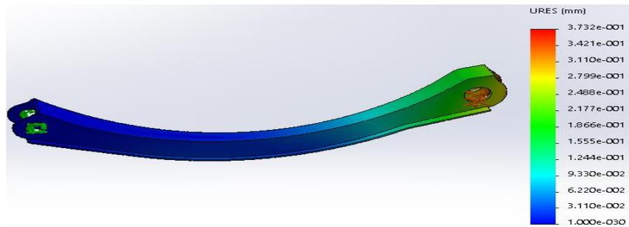
Fig. 16. Deformation for the modified design Rear Trailing Arm
