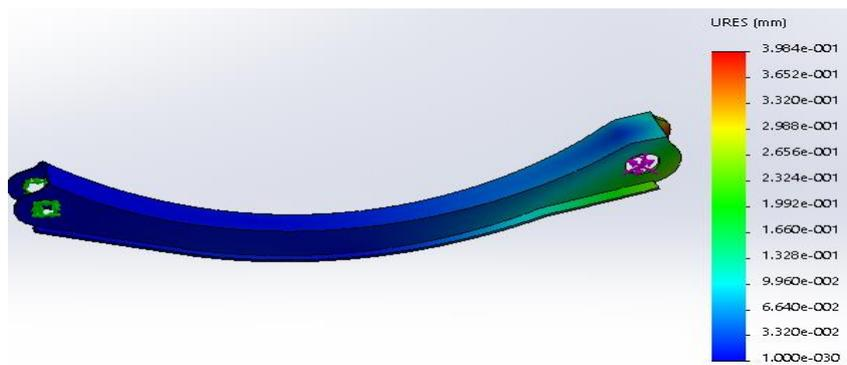
Fig. 12. Deformation for the existing rear trailing arm of 1G bump load
