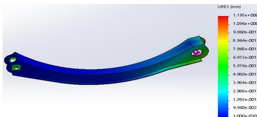
Fig. 14. Deformation for the existing rear trailing arm of 3G bump load
