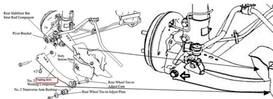
**Fig. 4.** Diagram of trailing arm taken from operational manual of Geely Addis
