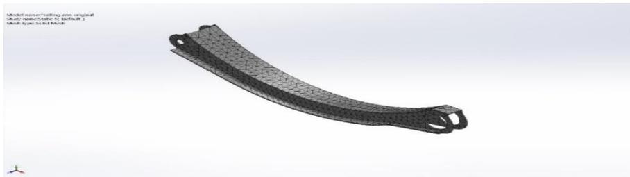
**Fig. 8.** Meshed existing Rear Trailing Arm
