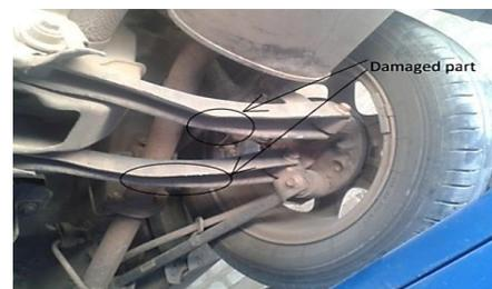
**Fig. 2.** Damaged trailing arm under maintenance
