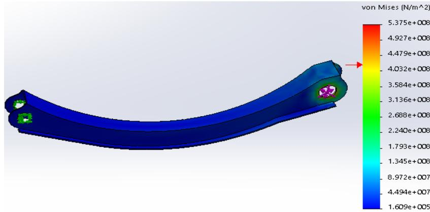
Fig. 11. Von mises stress for the existing Rear Trailing Arm of 3G bump load
