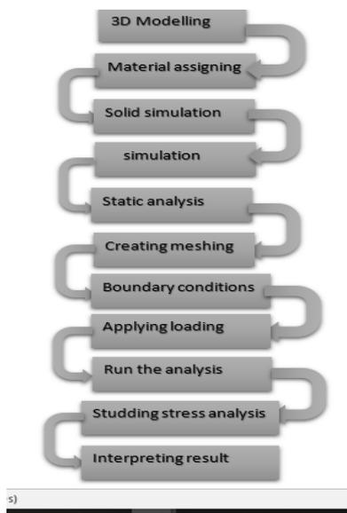
**Fig. 21.**Diagram of analysis procedure
