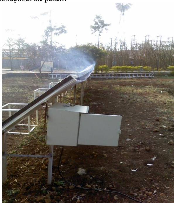
Fig 20: Smoke Flow Visualization Test
