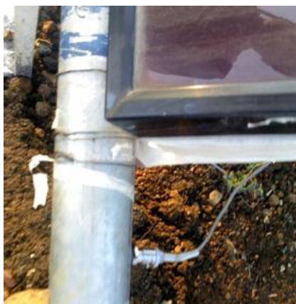
Fig 19: Thermo couple arrangement
