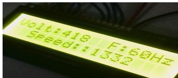
Fig. 11: Snapshot of three-phase output voltage displayed in LCD.
