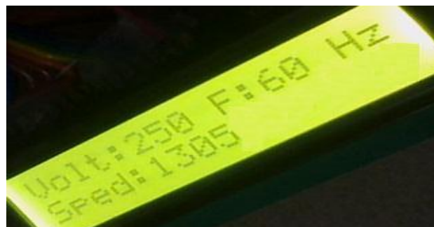
Fig. 10: Snapshot of LCD displaying single-phase boosted voltage and speed of the induction motor.
