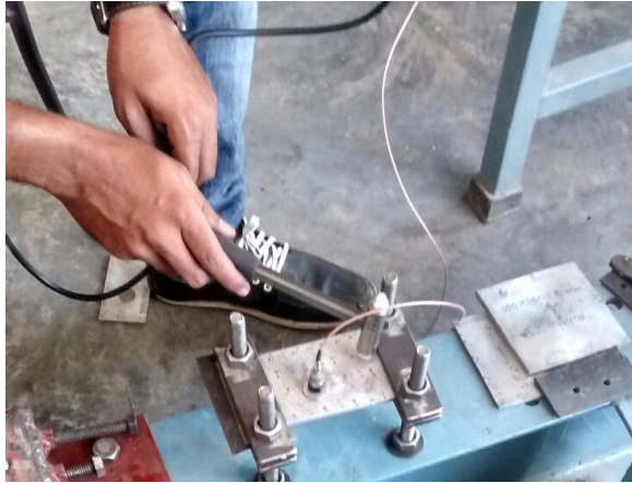
Fig.5 Experimental modal test
