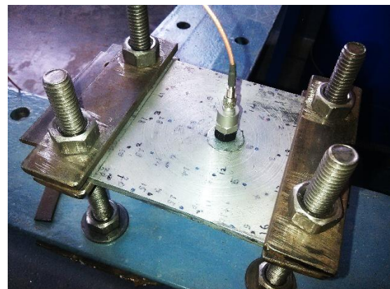
Fig.4 Plate fixed with CFFF condition
