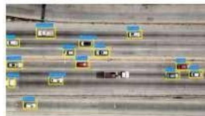
Figure 4: The use of DeepSORT for the tracking of vehicles
