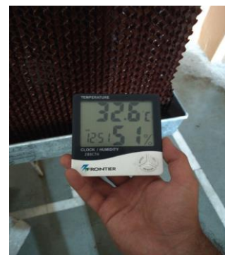
Figure 7 Measurement of RH using Digital Hydrometer
