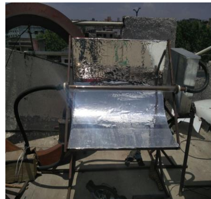
Figure 6 Parabolic Solar Collector
