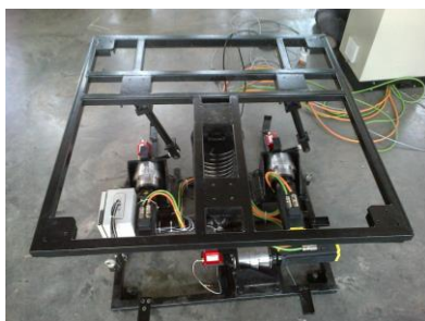
Fig.3 Setup of 3DOF Motion Platform
