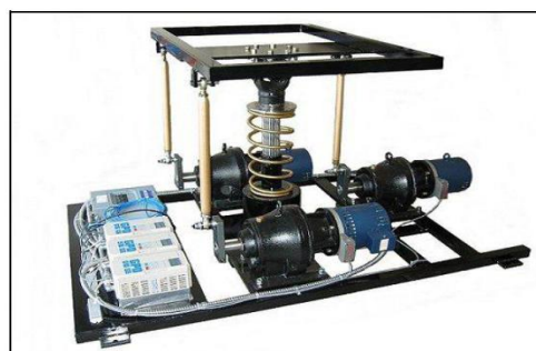
Fig.1 3-DOF and 6-DOF Motion Simulation Platform
