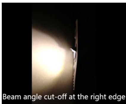
Fig.6 Beam angle cut off
