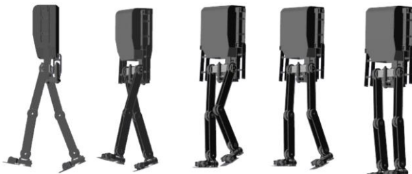
Fig. 13. Modeling of the Archie Robot in SimMechanics
