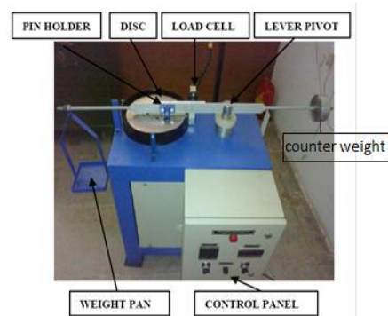
Fig.2 Pin on disc Test-Rig
