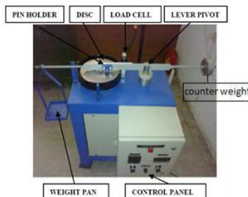
Fig.2 Pin on disc Test-Rig
