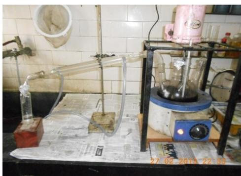
Fig.1 Transesterification setup
