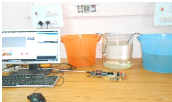
Fig.6 Snapshot for complete system of level measurement and control using ultrasonic sensor
