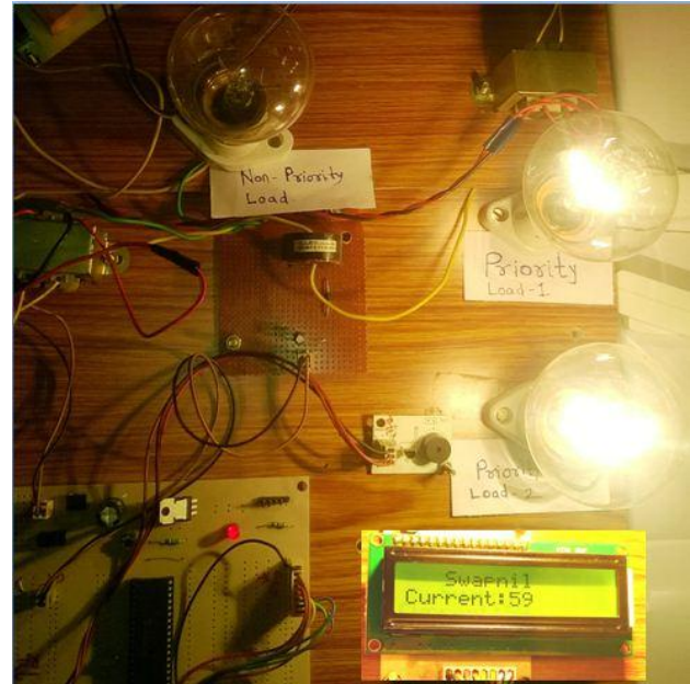
Fig.10. Stable system after non-priority load Trimming
