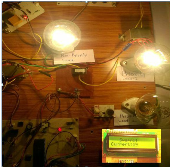
Fig.8. Full load condition of Transformer
