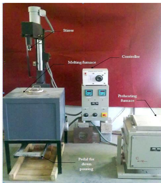
Fig. 1 Stir Casting - laboratory setup
