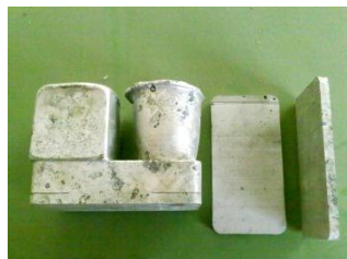
Fig. 3 Typical Al MMC casting along with machined plates
