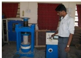
Fig.7 Comp. Test on cylinder
