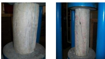
Fig.8 Failure of cylinder specimen
