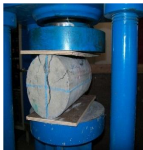
Fig.15 Failure of Specimen
