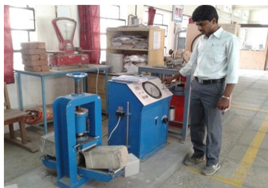
Fig.10 Testing of beam specimen
