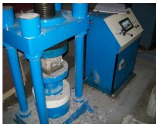
Fig.4 Testing of cube specimen
