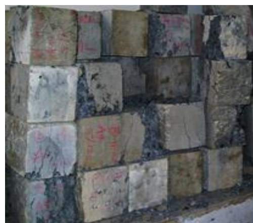
Fig.5 Failure of cube specimen
