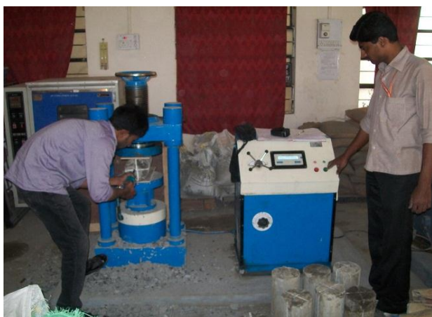
Fig.13 Testing of cylinder specimen
