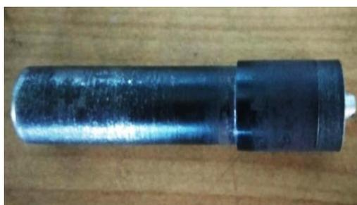
Fig 2 Friction stir welding tool (H13)
