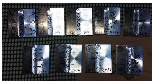
Fig 3 Friction stir welded pieces
