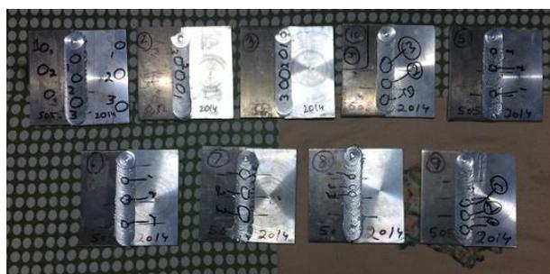
Fig. 3 Positions of penetration of nib ball on welded joints for testing hardness
