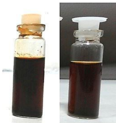
Figure 5 The photos of dispersion of Cunps (A) before (B) after 2 months of storage
