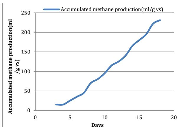
**Figure 4:** Accumulation of methane production from digester 3
