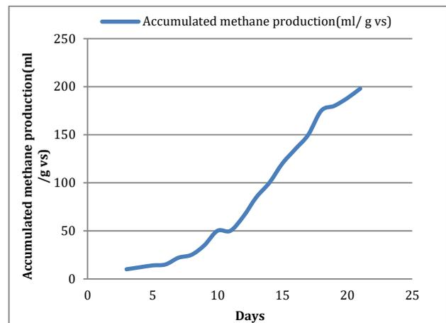
Figure 2: Accumulated methane produced from digester 1
