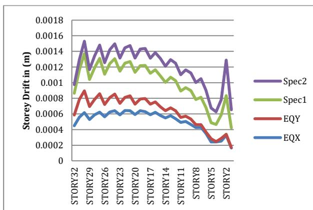
Fig.3 Storey VS Storey Drift – X Direction (m)
