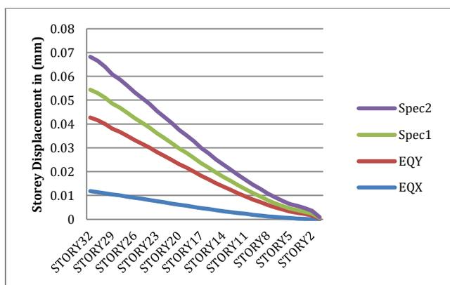
Fig.6 Storey VS Displacement- Y Direction (mm)
