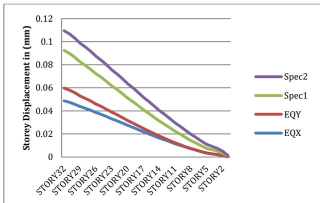
Fig.5 Storey VS Displacement – X Direction (mm)
