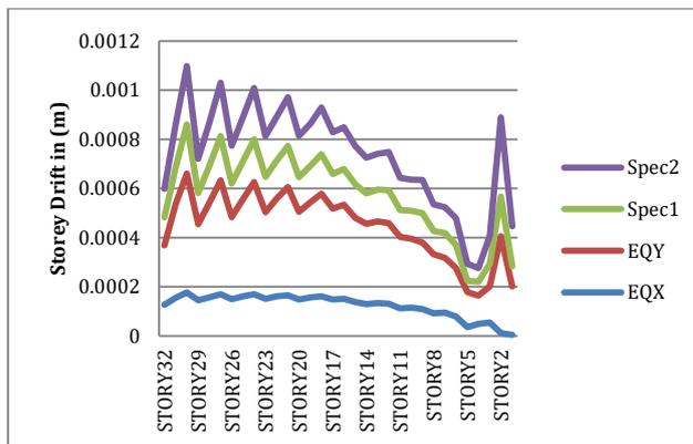
Fig.4 Storey VS Storey Drift – Y direction (m)
