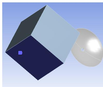
**Fig. 5:** Fixed support to the bottom side of the soil body
