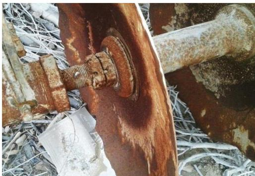
**Fig. 2:** Erosion of Disk Harrow
