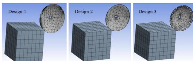
**Fig. 4:** Meshing view of all designs of disk harrow
