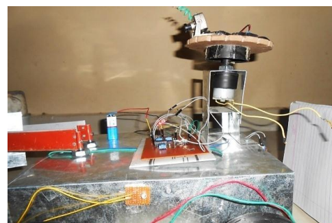
Figure 12: Results of the obstacle detection circuit
