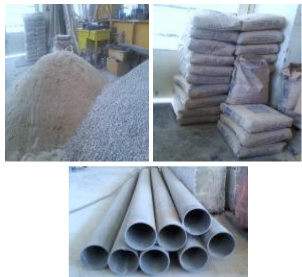
Fig. 2 Cement, Gravel, Sand and PVC Pipe Used
