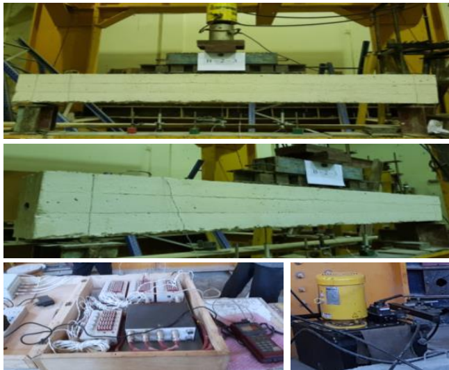
Fig. 7 Beam Test Setup, Dial Gauge and Load Cell
