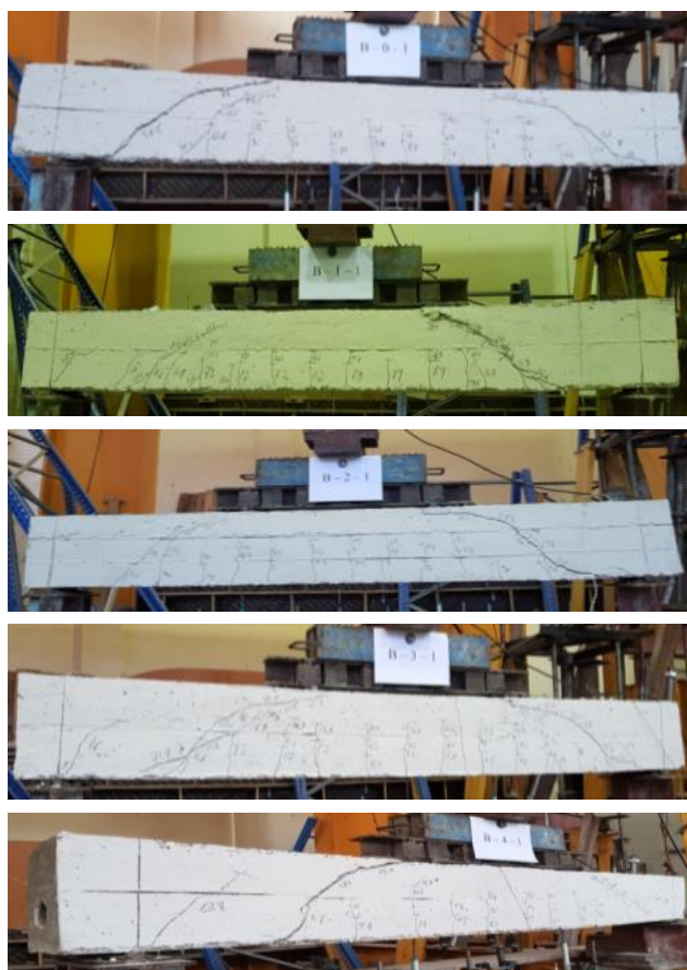
Fig.12 Crack Pattern for Beams with Under Reinforced Section
