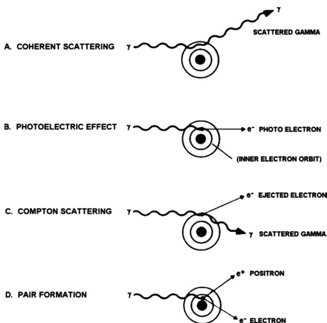
**Figure 1.** Schematic description of the four main processes accounting for  $\gamma$ -ray interaction and absorption [book].
