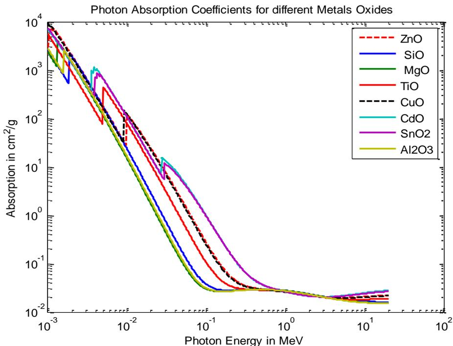
Figure 3. The total mass absorption coefficients for the evaluated metal oxides
