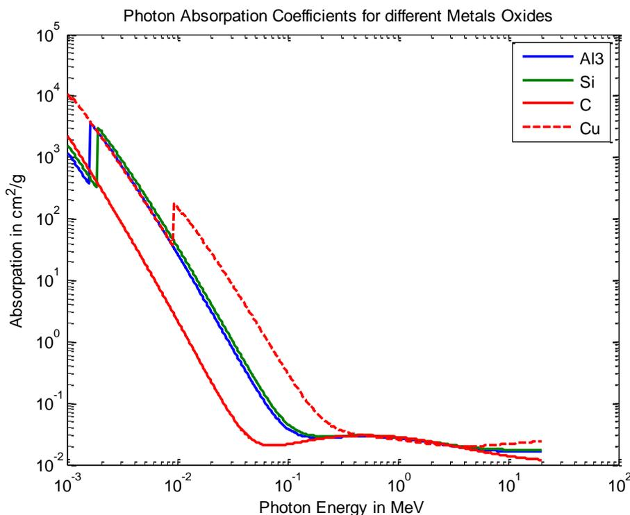
Figure 4 Total mass attenuation coefficients for the evaluated metals.
