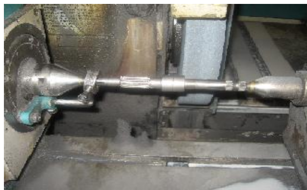
Component clammed on slot side
