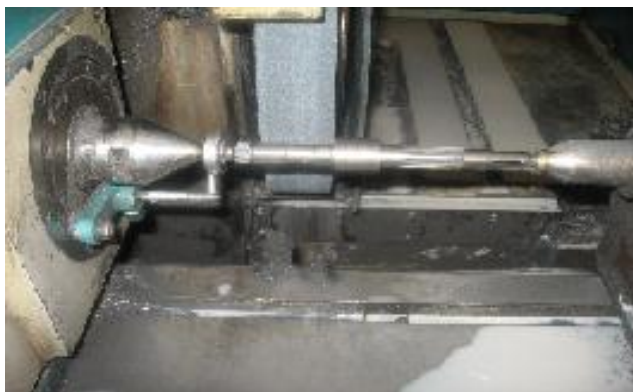
Component clamped on serration side.
