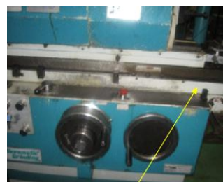
After Dressing of grinding wheel, wheel location manually set by operator
