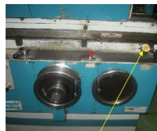
Dial provided on grinding machine slide to set the proper location of grinding wheel after the wheel dressing
