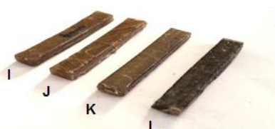
Fig.3 RPET samples with different melting temperature I-at 180 °C, J-at 200 °C, K-at 220 °C and L- at 240 °C for charpy impact test
