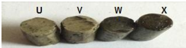
Fig.6 RPET samples with different melting temperature U – at 180 °C , V –at 200 °C ,W –at 220 °C and X –at 240 °C for wear test
