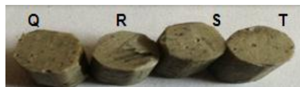
Fig.5 RPET samples with different melting temperature Q– at 180 °C , R –at 200 °C ,S –at 220 °C and T –at 240 °C foe wear test
