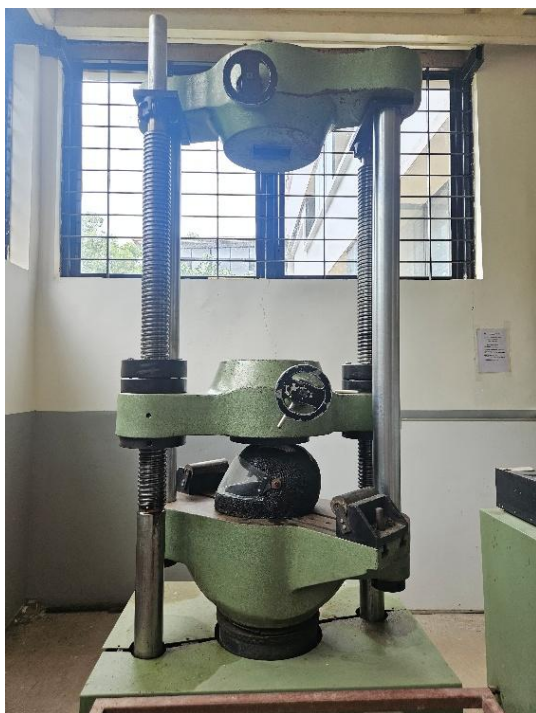
Fig. 5 Compression Testing of Helmet using a Universal Testing Machine
