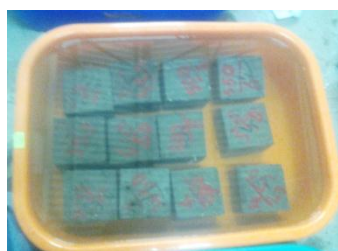
Fig 3 Sulphate attack test
