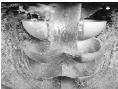
Fig. 3 External stroboscopic view of pelton turbine. (A. Rossetti et al, 2014), (G.Pavesi et al, 2014), (A.Santolin et al, 2014)
